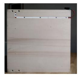
This is the bottom of the vault. Their is a trench for the power supply to travel from the back of the vault to the door inside the vault.
