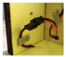
When assembling the door, connect the power supply cable to the door cable.
